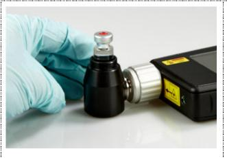
When the vial is in position a part of the vial will be raised above the vial holder and it is not possible to screw on the cap of the vial holder.
